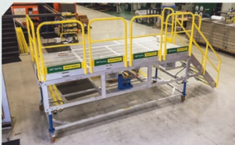
▲ Large rolling platform with single point hydraulic adjustability
