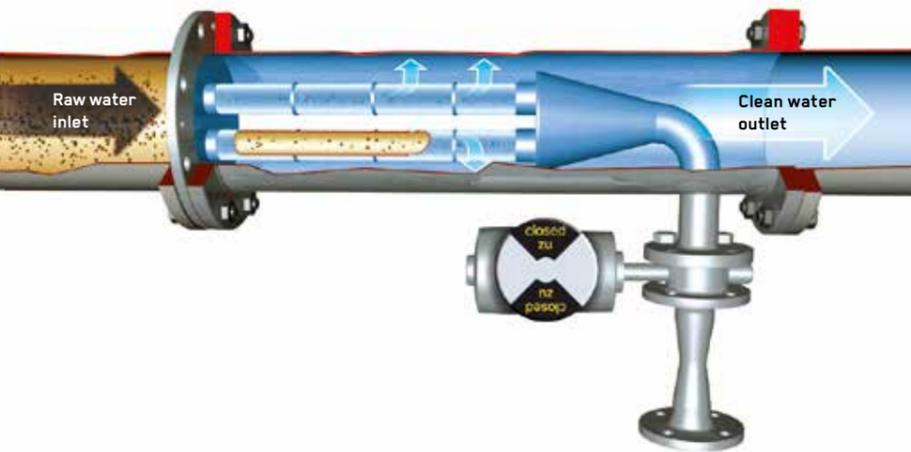
The raw water flows through the openings in the clamping plate, entering the filter elements located behind them. The reductions in cross-section result in a proportional increase in the axial flow velocity in the filter element of 5-7 m/s. A conical dirt collector is located at the end of the filter elements, joining these together.
