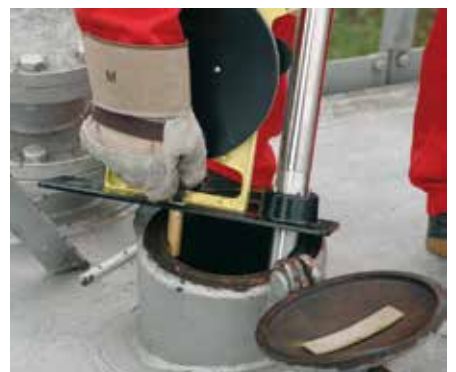
for gauging pipe up to 6 inch diameter
