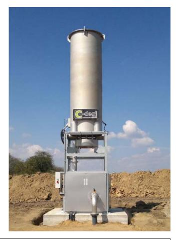
Type: Combustion capacity: Equipment: LTC, biogas emergency flares 50 kW – 20 MW (or more, on request) enclosed combustion (flame not visible), integrated ATEX blower, gas train enclosure
