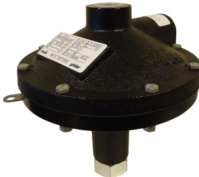
The 275 D relief valve is installed downstream of pressure regulators to relieve limited volumes of gas. Used where venting to the atmosphere is acceptable, it provides a cost-effective solution to prevent safety shut-off valves from triggering in case of thermal expansion, transient pressure surges and creep leaks from regulators. This valve is ideal for low pressure settings due to the increased sensitivity provided by a large diaphragm area.
